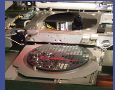
DBI™ pick & place placement accuracy is +/- 1μm over 3σ.
